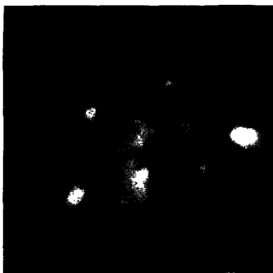
FIG. 5. Microdiffraction pattern from faulted Au crystal in [111] orientation showing weaker net of "forbidden" reflections.
