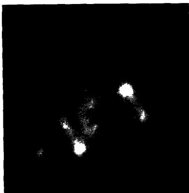
FIG. 7. Pattern from heavily disordered crystal, thought to be Ru with disorder of layer stacking.
